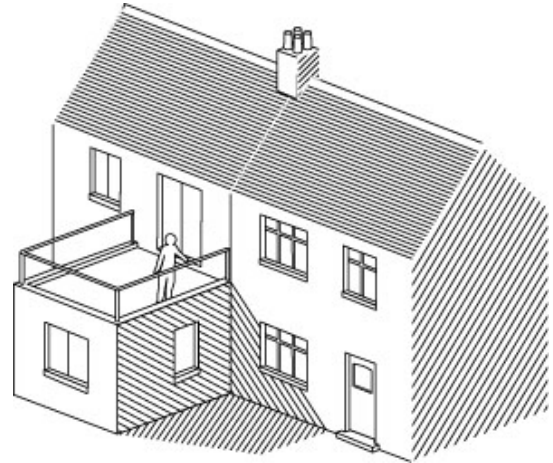
Fig 1. Overshadowing, overlooking and loss of outlook
